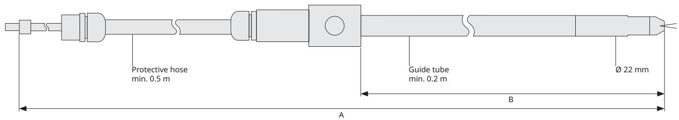
D-LL 703 | FLEXIBLE FIBRE OPTIC SYSTEM FOR D-LE 703, D-LX 701, D-LX 710 AND D-LX 721
