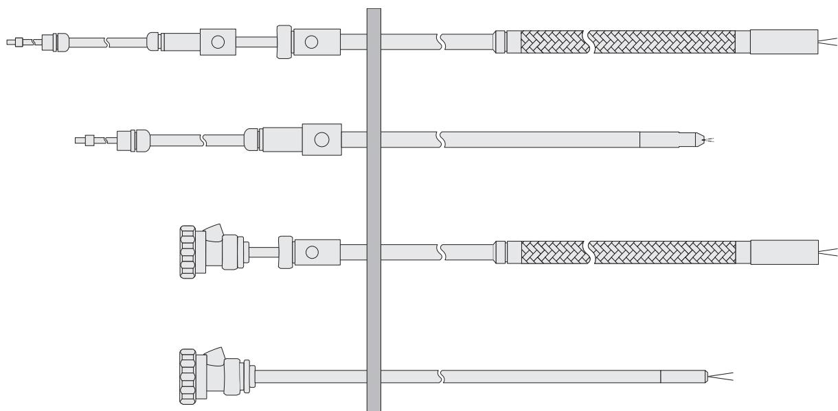
D-LL 701 | FLEXIBLE FIBRE OPTIC SYSTEM FOR D-LE 701
